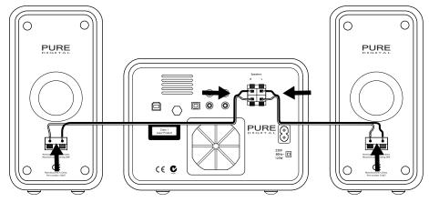
When connecting speakers connect the red (positive) terminals on Legato to the red terminals on the speaker and black (negative) to black. The speaker cable has a stripe on one strand to aid connection.
